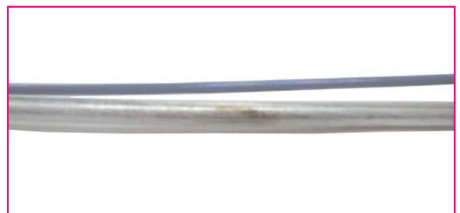
Aluminium cables suffer far less damage when exposed to an identical lightning strike. No damage is caused to the inner aluminium tube or the fibre.
