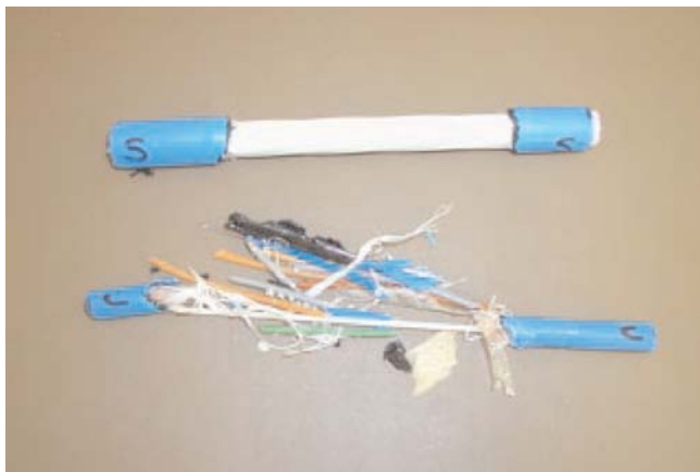
Rodent attack comparison: Severest attack examples. ARM@CORE (S) vs. Conventional Loose Tube Cable (C)
